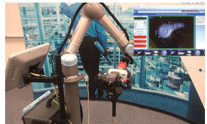
Cobot visually inspects a part to ensure certain features are present.
