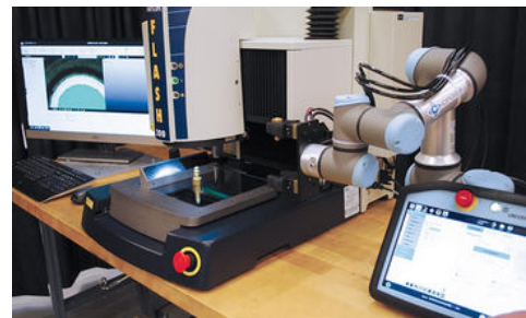
Cobots can be programmed to communicate directly with video measurement equipment, allowing them to place parts and then sort parts based on the data collected.
