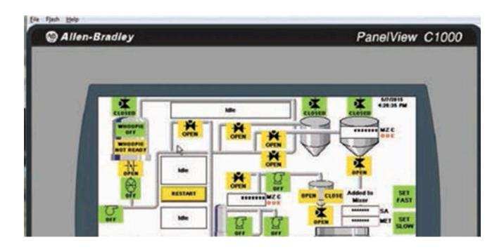
First, soda ash is blown through a three inch feed line to weigh hoppers on the roof and then measured into the mixer. The second ingredient, metso powder, is held in a large container on load cells. It operates by measuring the loss in weight, so powder is sucked into the mixer until the weight drops by the amount called for in the recipe.
