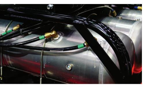
leads to a poor seal: The process requires female threads to be machined into steel spuds that are welded into the air tank. The ensuing welding process can cause the spuds to warp, which results in a poor fit.
