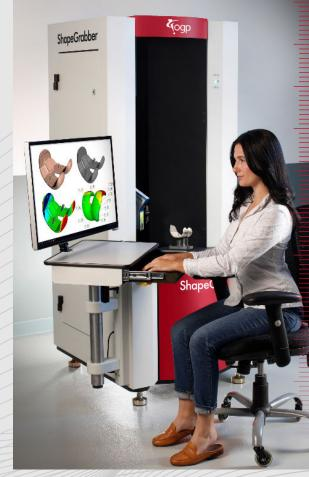
ShapeGrabber 3D scanners are ideal for quality control as they allow you to rapidly measure and inspect complex parts. Our industrial scanners provide 3D scan data using a fraction of the time and resources compared to more traditional methods.
