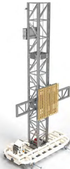
Fully constructed, the solar simulator tower reaches three stories. Here, the pantographic morphing array is shown in its six-by-six-foot configuration.
