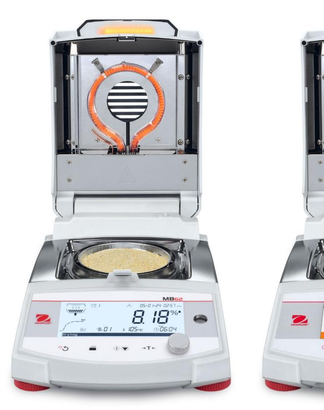
The MB62 is versatile and suitable for a variety of moisture applications across different industries.
