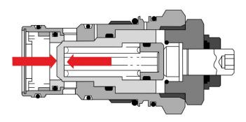
it is applied to the valve port of the counterbalance valve. To overcome the added pressure on the valve port, the part balanced 1CER references the added pressure to the spring chamber. This pressure is now acting on both ends of the poppet and becomes balanced or negates the effect of the backpressure on the valve port.
