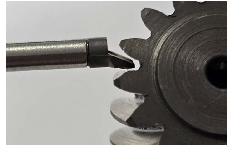
A skidded probe is too large to be able to measure down to the root of the tooth.
