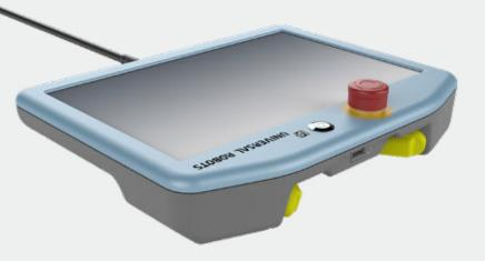
A 3-position enabling teach pendant is now available as a variant for all payloads of UR robots, and as a UR+ component. The 3PE device is mechanically and functionally integrated with the Teach Pendant – just plug-and-play with any control box. Additionally, it is fully integrated into the Polyscope user interface to enable all robot motion, including Freedrive, in manual mode.
