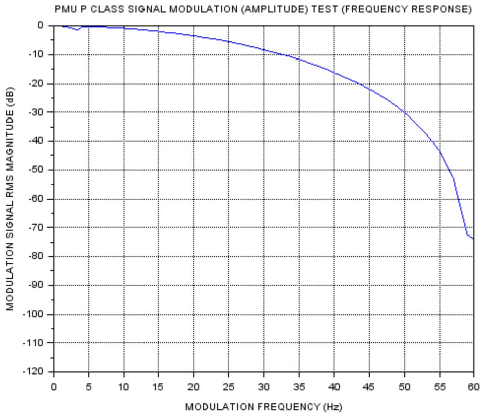
**Fig.4:** Modulation signal magnitude vs modulation frequency for the P class reference design
