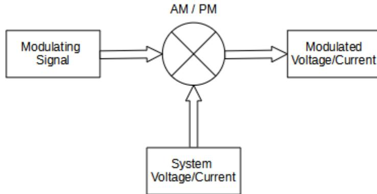
**Fig.1:** Amplitude/Phase modulation (AM/PM) to emulate power system oscillations
