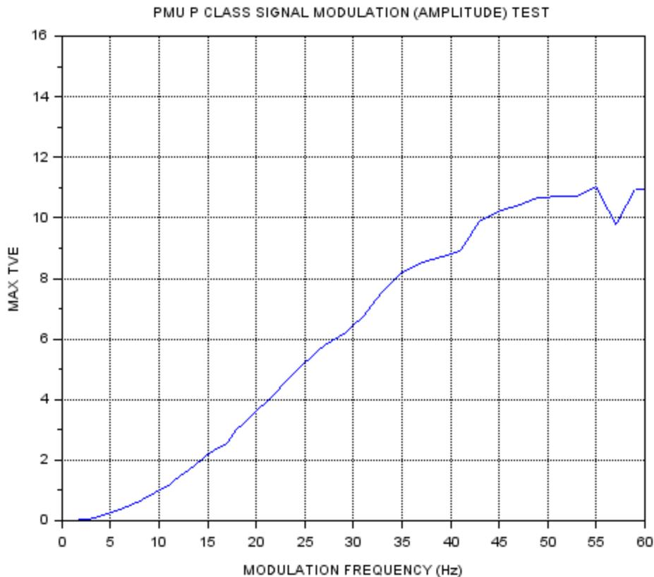
**Fig.3:** TVE vs Modulation frequency plot for the P class reference design (0 – 60 Hz)
