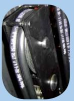
Products in this brochure have been well tested in the most extreme applications by Parflex and our customers. Even in the severe temperatures of industrial freezers, 53DM hose continues to perform at -70°F. A typical 53DM-6 meets SAE 100R18 and withstands more than 250,000 cycles in our freezer over the sheave test stand.
