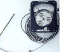
length of the temperature probe and the fact that the entire probe is part of the sensing element, finding the right equipment to calibrate correctly is essential.
