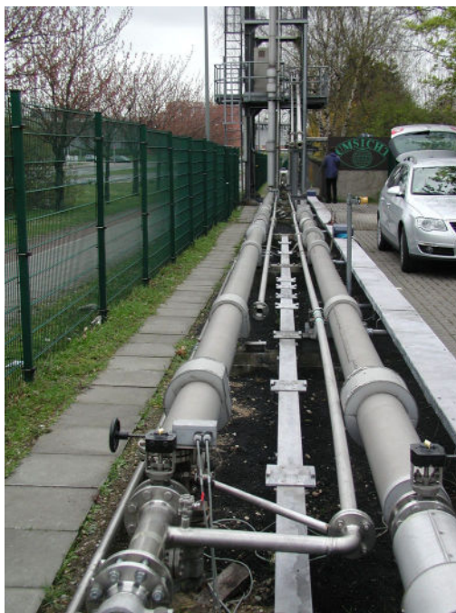
Fig. 11: Water hammer is doubled with a branch line [7]
