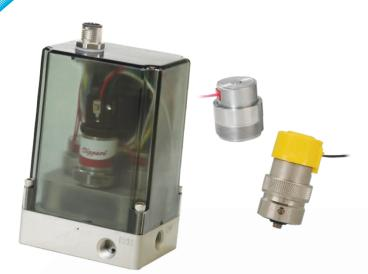
The Cordis CHP series utilizes Clippard's EHV and EHS lines of high pressure electronic valves to allow for steady, repeatable downstream pressure under static conditions. The result is precise, linear pressure control within a closed loop system.
