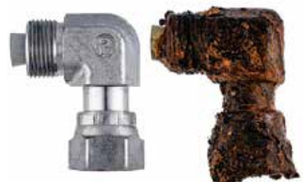
ToughShield Plus (left) and Zinc-crimped (right) swivel adapters after 3,000 hours SST
