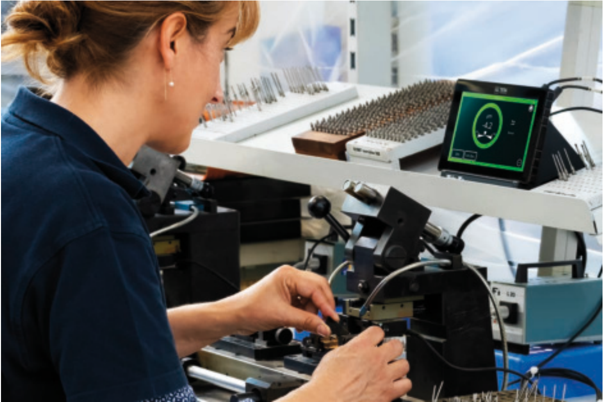
Concentricity measurement before assembly of cylindrical parts
