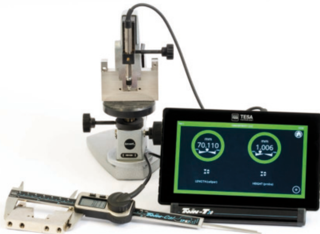
Control of 2 functional measurements, one with a TESA inductive probe and the other with a calliper connected to the display.
