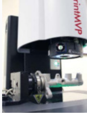
Optional rotary indexers automatically index parts for complete measurement of all features.
