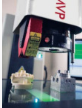
Optional DRS laser and touch probe offer additional sensor capability for complex measurements.
