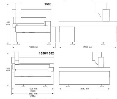
System Weight: 1500 Model: 2,590 kg 1550 Model: 5,460 kg 1552 Model: 6,380 kg Shipping Weight: 1500 Model: 3,000 kg 1550 Model: 6,260 kg 1552 Model: 7,280 kg
