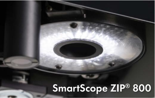
**SmartScope ZIP 800** is designed for applications involving larger, heavier parts. Optional 300 mm Z-axis travel provides additional measuring volume. ZIP 800 also offers:
