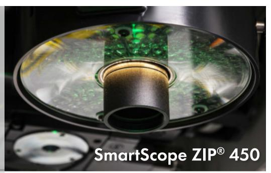
**SmartScope ZIP 450** is a floor model metrology system offering video and multisensor measurement for large parts. It has a reputation for extreme reliability and proven metrological performance. The ZIP 450 also offers:
