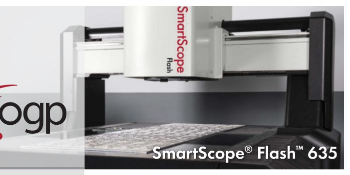
SmartScope Flash 635 – Provides measurement speed and stability in addition to an ergonomic loading height. The rigid drive system contributes to long-term reliability. The 635 features a moving bridge design where the part remains stationary. A granite base and extruded lightweight aluminum bridge provide measurement stability at high speed. Flash 635 offers:
