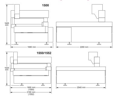
Flash 1500 System Weight: 2590 kg Shipping Weight: 3000 kg Flash 1550 System Weight: 5460 kg Shipping Weight: 6260 kg Flash 1552 System Weight: 6380 kg Shipping Weight: 7280 kg
