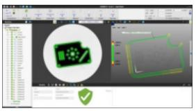
ZONE3 uses innovative features to automatically generate measurement routines resulting in faster programming and run times. Parallel Processing combined with intelligent routine Optimization can be used to measure as many features as can be seen simultaneously.
