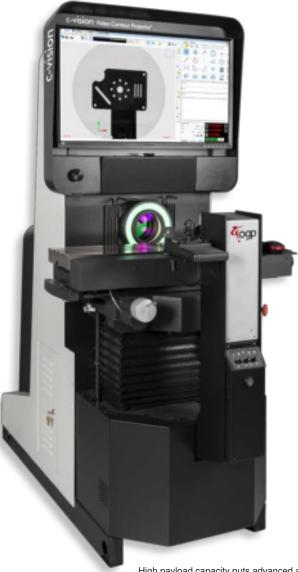
High payload capacity puts advanced automatic video measurement to work for large, heavy parts. Shown with optional LED ring light.
