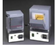
diameter port at the rear of the chamber allows insertion of an independent measuring device to monitor chamber temperature. Chambers have a volume of 76 (5300A01) or 129 cubic inches (5300A05). Chamber interiors measure 5" D x 3.8" H x 4" W and 5.6" x 4.9" x 4.7", respectively.
