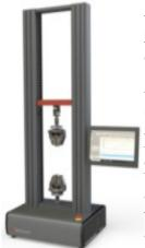
Fabrics are the end result of many complex procedures and there are many factors that can influence their final quality and performance. An effective way of monitoring fabric quality is to conduct tensile and related strength tests at various stages of production. Ensures that your fabric has the strength and integrity for its intended purpose.
