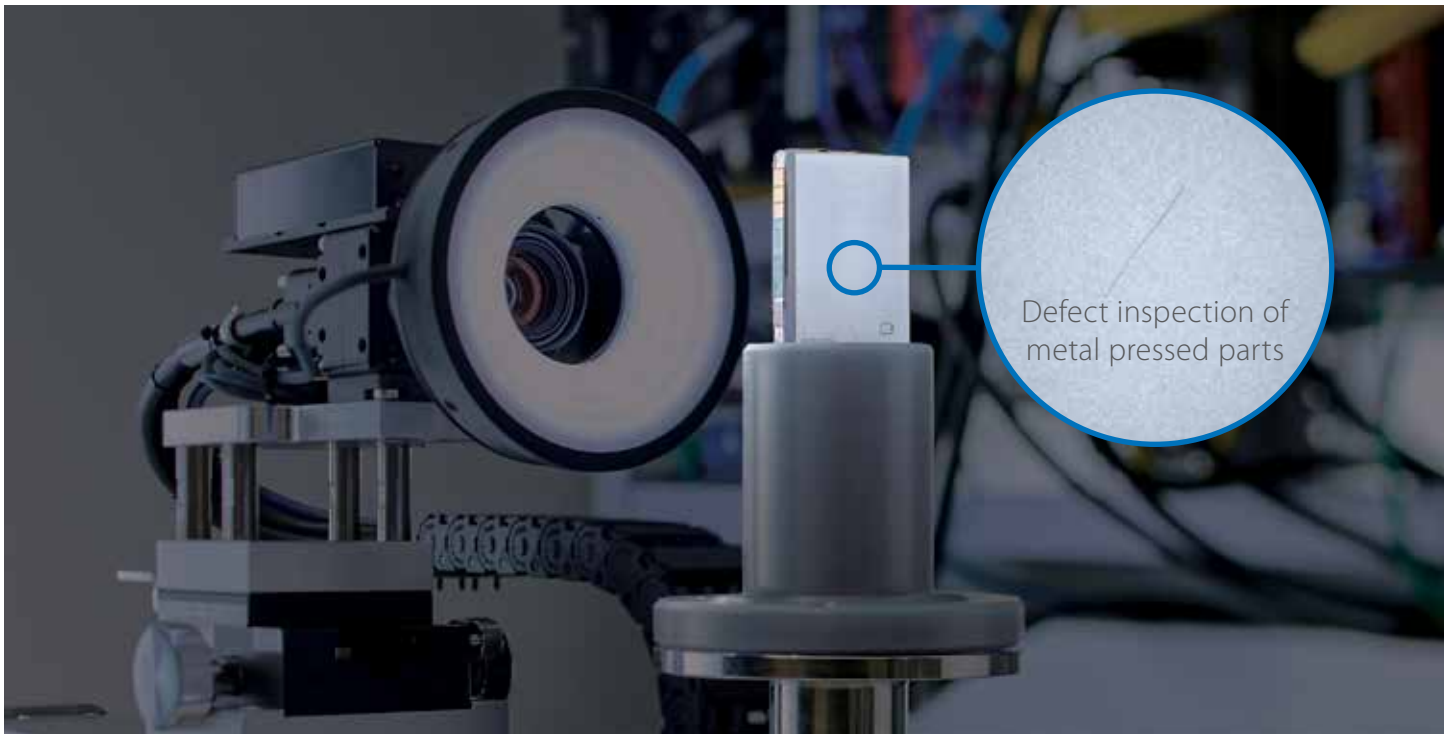
Automating human vision-based inspection with the FH Series
