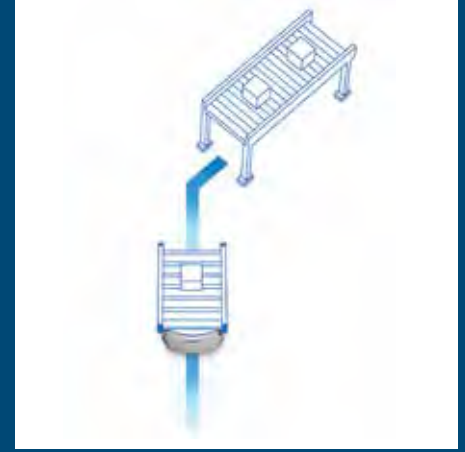
High Accuracy Positioning System (HAPS) HAPS allows our mobile robots to move along fixed paths in applications that require tight tolerances.
