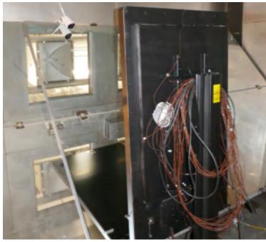
In order to properly test the monitors, they needed to be mounted upright, just as they would be when used in a normal application. Because the lights in the solar chamber are directly overhead, the testing engineers had to get creative. The team utilized mirrors to redirect the light radiation towards the front screen while maintaining the proper orientation for gravitational effects.
