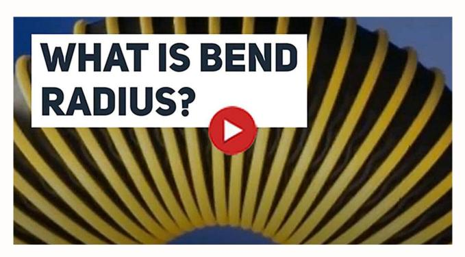
A hose's bend radius determines how long a hose needs to be before it can safely bend while in service. Understanding bend radius helps ensure a hose will have the necessary strength and functionality for its intended use case. Failing to account for bend radius limits will ultimately cause damage to hoses and shorten their usable service life.
