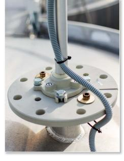
The equipped level transmitters are continuously measuring the level in the silos and transmit the measured values via HART protocol to the **MultiCONT** multichannel controller which transmits the data via RS485 communication line to a PC.
