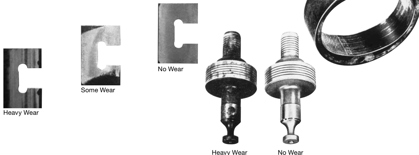
Figure 1. Typical Examples of Wear Due to Contamination
