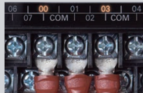
Input/output terminal LED indicators for quick troubleshooting
