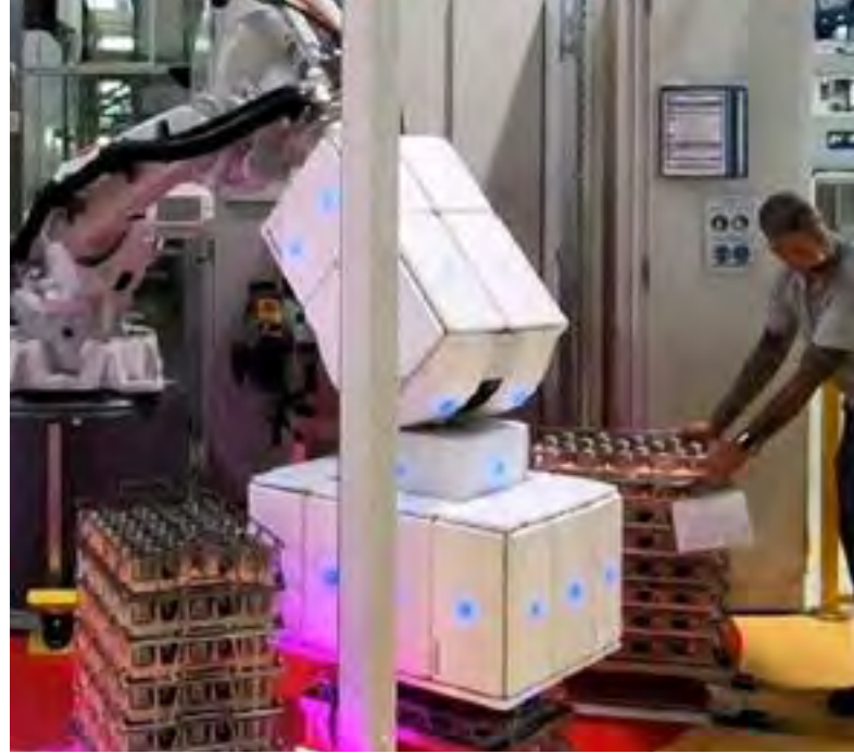
AIRSKIN® at MAGNA production plant ABB robot and custom gripper with AIRSKIN® modules
