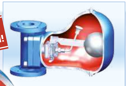
Extra-high performance version for condensate volumes > 10,000 kg/h and differential pressures up to 32 bar. Robust lever and ball design
