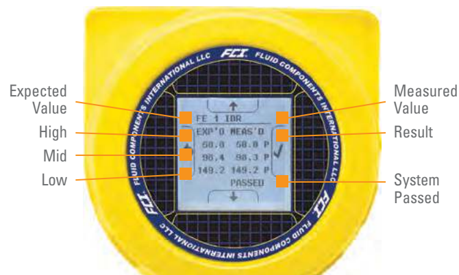
Figure 1. Front panel; all three check points show "P" (pass) and entire self-check "PASSED"
