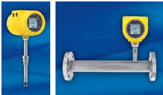
Model ST80 (left) is an insertion flow meter for pipe sizes from 2 1/2" to 99" [64 mm to 2500 mm]. Typical calibration range is from 0.25 SFPS to 1000 SFPS [0.07 NMPS to 305 NMPS].
