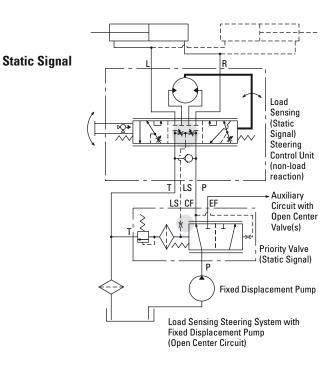
Work Circuits: Non-Load Reaction and Load Reaction
