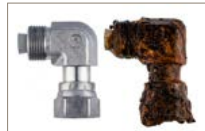
Figure 9: ToughShield Plus (left) and Zinc-crimped (right) swivel adapters after 3,000 hours SST
