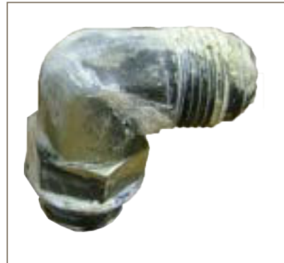
Figure 5: Zinc Oxidation on a Steel Tube Fitting
