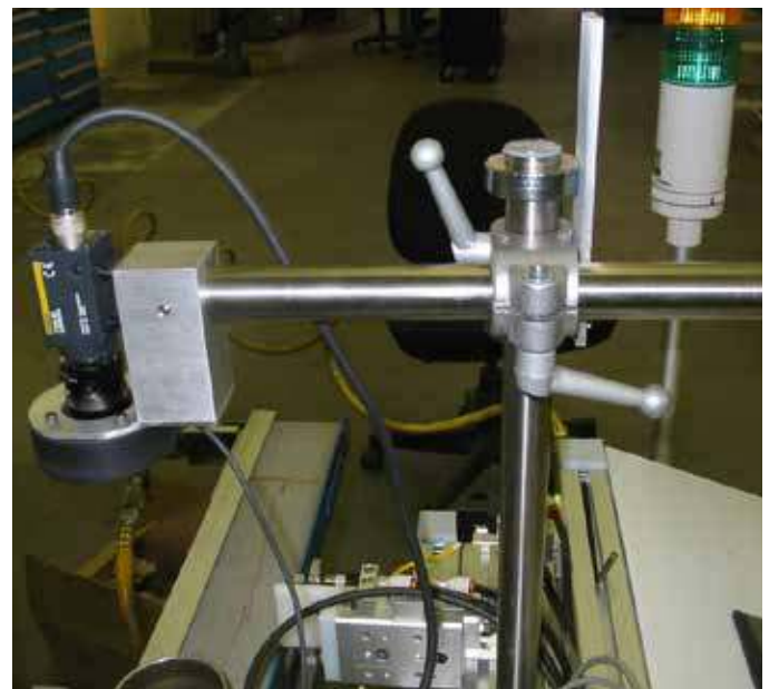
The camera and the low-angle ring light are mounted above the conveyor, with the camera's position capable of being manually adjusted in two directions.
