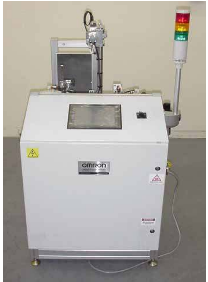
The Can Flange Inspection System's front view shows the control panel and the operator panel.
