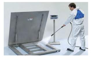
this solution, the entire scale tilts up 45 degrees, exposing all surface areas for cleaning. An automatic safety system restrains the platform if pneumatic pressure is lost. The pneumatic controls typically can be locked to prevent unauthorized personnel from operating the system.
