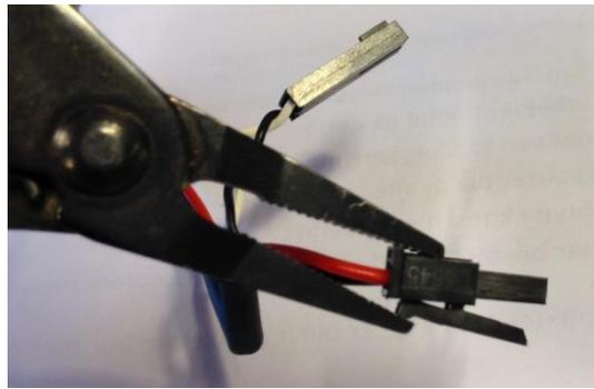
4. After disconnecting the wires gently remove black flexible flat ring with a tiny screwdriver and twist it around the joint housing.
