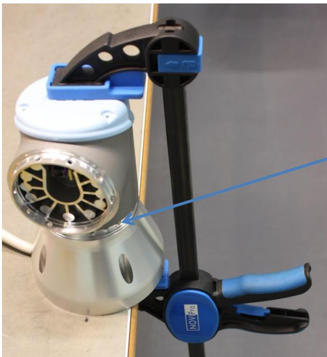
6. Gently tighten the 10 screws, and then tighten **in cross order with 3.0Nm**.
