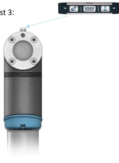
Wrist 3 zero position is aligned so tool connector is pointing upward. Mount two bolts in tool holes and use spirit level to align joint.
