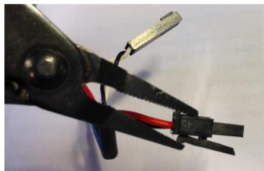
7. After disconnecting the wires gently remove black flexible flat ring with a tiny screwdriver and twist it around the joint housing.
