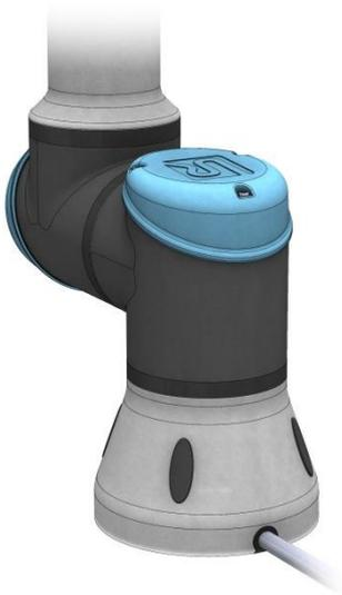
Base zero position is aligned so that the output flange is offset 180 degree from the slot for cable in back of robot base.
