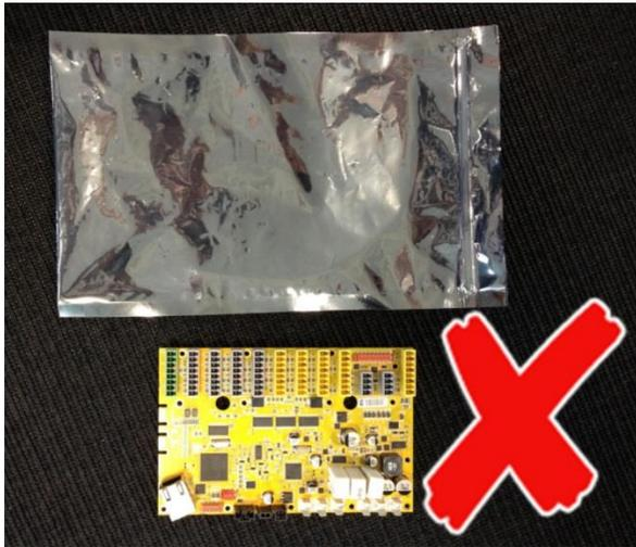
**Do not** place the ESD-sensitive part on nonconductive material or on a metal table.
