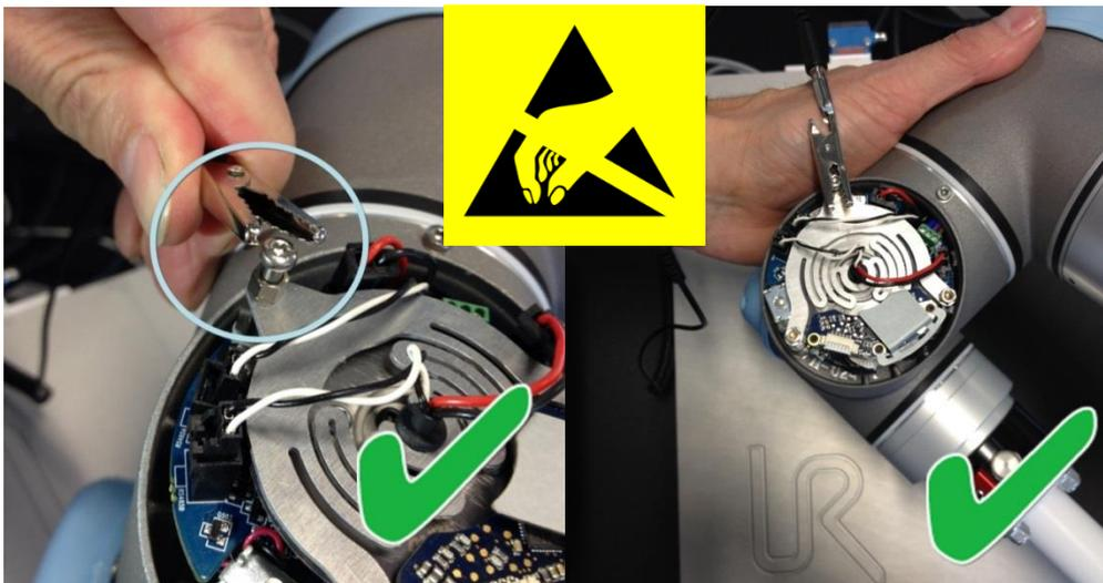
6. **Gently** unplug the cable connectors **without bending the printed circuit board**.
