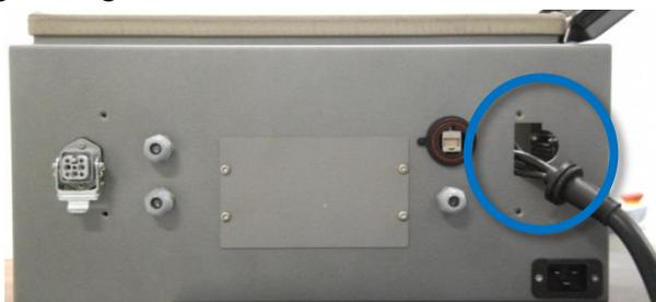
3. Replace teach pendant with new, insert cable in cable inlet and perform reconnection of all plugs and mounting of aluminum cover in reverse order to the above description.
