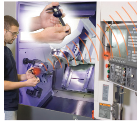
▲ Integrated Wireless is ideal for point of manufacture inspection, making measurements directly in the machine with immediate feedback to the machine controller.
