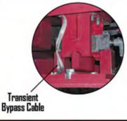
**Wire Braided Copper Transient:** By-pass cables at each load cell mount help route surges around the load cell to ground rather than through it. The number one cause of load cell failures are lightning strikes that travel through the weighbridge and load cells, damaging load cells.
