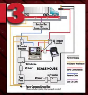
**Lightning Protection:** Every Rice Lake Truck scale comes complete with a Surge Voltage Protection System that includes a UPS 2000 Sola Duplex Transformer. The junction box is provided with individual UJB-3T6 DC transient circuitry protection. The entire system is grounded to a single-point grounding system connected to the power ground. Our scales come with a Five-Year warranty on the load cells and junction box, and Five-Year warranty on the weighbridge.
