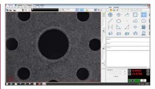
Transform the traditional optical comparator into a fully automatic inspection system with optional VidiProbe and SNAP-X<sup>™</sup> software. The video camera is internally mounted to enable simultaneous measurements using both the analog comparator screen and the digital video with SNAP-X.
