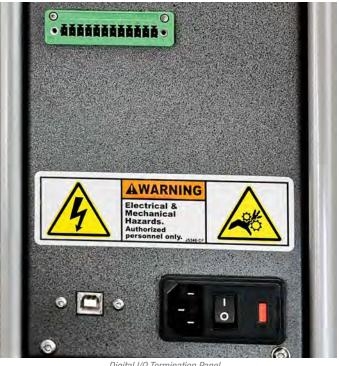
Digital I/O Termination Panel Shown on FMS and FMD Force Test Frames (FMS5000)
