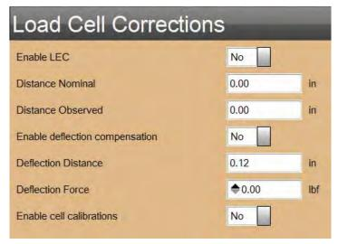
L3 LOAD CELL CORRECTIONS Setting Used for calibrating load cell sensors and test frame
