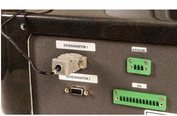
Analog and Digital I/O Termination Panel Shown on MMS and MMD Material Test Frames (MMD-50K)
