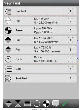
L2 Plus Test Stage Shows multiple step test setup
