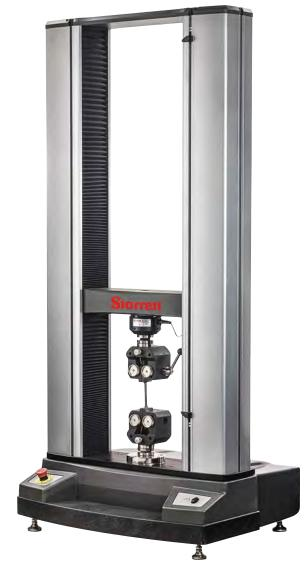
FMD-50K Series Testing Frame (50kN, 5000 Kgf, 11,250 lbf)
