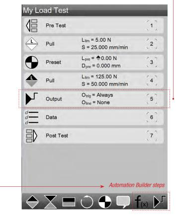
L2 Plus Graph Analysis Tools Shows optional formula tool with Automation Builder option installed
