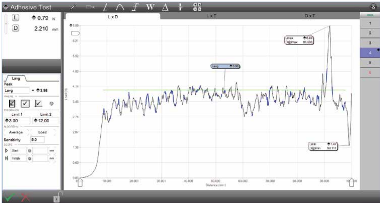
Full Graph of Adhesive Peel Test Displays Maximum and Minimum load values plus average of qualified Peaks using Sensitivity adjustment
