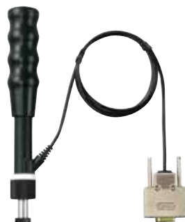
810-289 Use for concave workpieces such as gear teeth, ball bearing races, etc.
