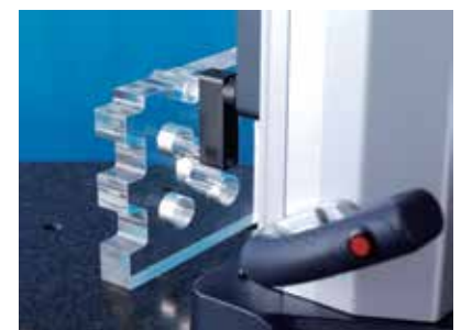
Inside diameter measurement
