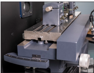
Helix Stage Motion allows the worktable to pivot for gear and thread measurements.
