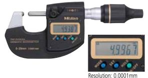
The High-Accuracy Digimatic Micrometer utilizes Mitutoyo's innovative  $0.1\mu m$  resolution ABS (absolute) rotary sensor and high-accuracy screw machining technology to reduce the instrumental error to  $\pm 0.5\mu m$ , delivering higher accuracy  $(0.1\mu m)$  without sacrificing operability.
